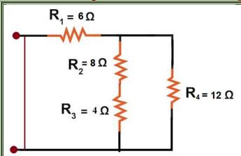
Two resistors  $R_2$  and  $R_3$  are in series
