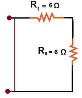
Two resistors  $R_1$  and  $R_6$  are in series
