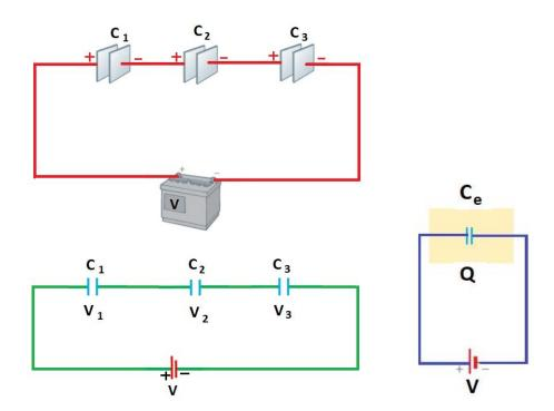
When a battery is connected to the circuit, electrons are transferred from the left plate of  $C_1$  to the right plate of  $C_3$  through the battery. The result of this that all the right plates gain of negative charges of -Q and all the left plates have charges of +Q.
