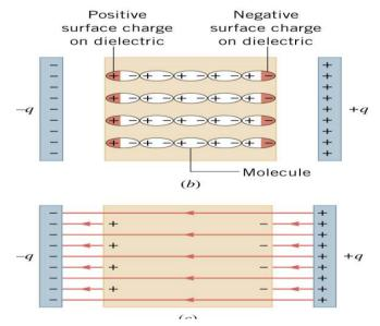
Due to this polarization the potential on plates decreases and a capacitor connected to battery accumulates more charge, hence its capacitance increases.
