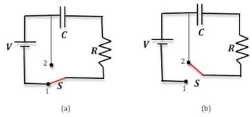
When a switch is at position 1 as shown in figure (a), the capacitor begins to store charge. If any time during charging, the charge Q flowing through a circuit and Q is the charge on a capacitor, then sum of the potential difference between the palate of a capacitor and across the resistor is equal to the potential difference from the battery. As the current stop flowing when the capacitor is fully charged, when  $Q = Q_0$ , then
