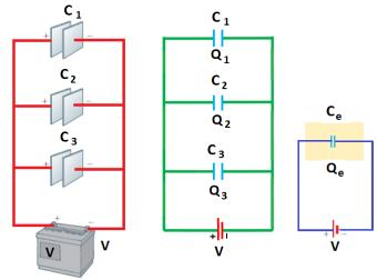
The individual Potential difference across capacitors connected in parallel are all the same and are equal to the potential difference applied across the combination. Now,
