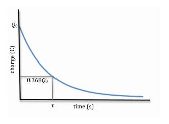
Time constant of RC circuit is thus also the time during which the charge on the capacitor falls from its maximum value to 0.368 of its maximum value.
