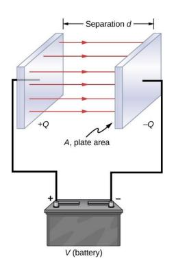
That is, the capacitance of a parallel-plate capacitor is proportional to the area of its plates and inversely proportional to the plate separation.
