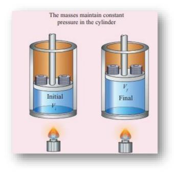
When the gas is heated at certain amount of heat energy is transferred into the system. The gas expands and move the piston outward, temperature changes from  $T_1$  to  $T_2$  and volume changes from  $V_1$  to  $V_2$ . If the displacement is kept very small, the pressure of gas will not be changed much and can be considered constant.
