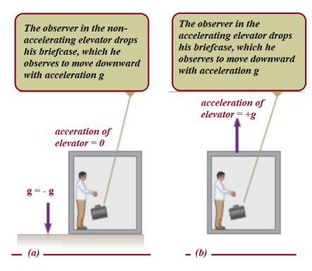
In each situation, an object released by the observer undergoes a downward acceleration of magnitude g relative to the floor. In Figure (a), the person is at rest in an inertial frame in a gravitational field due to the planet. In Figure (b), the person is in a no inertial frame
