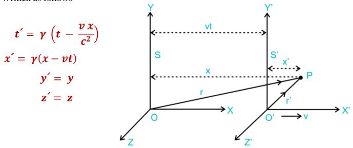
where t and (x, y, z) are the time and space coordinates in the original frame, t' and (x', y', z') are the time and space coordinates in the frame moving with velocity v relative to the original frame as shown in Figure, c is the speed of light, and  $\gamma = \frac{1}{\sqrt{1 - \frac{v^2}{c^2}}}$  is the Lorentz factor.
