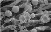
4. **Energy-Dispersive X-ray Spectroscopy (EDS):** With EDS detectors, electron microscopes analyze elemental composition by detecting X-rays emitted when high-energy electrons interact with the sample.
