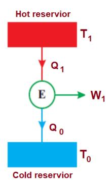
Consider an irreversible process, in which heat Q in a reservoir at temperature  $T_2$  ( $T_2 < T_1$ ). Let the temperature of the coldest available reservoir be  $T_0$ . A Carnot
