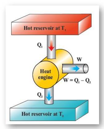
The engine itself is represented by the circle. The amount of heat supplied  $Q_1$  to the engine by the hot reservoir is proportional to the cross-section of the incoming pipeline at the top of the diagram. The cross-section of the outgoing of the pipeline at the bottom is proportional to the magnitude  $|Q_2|$  of the heat discarded in the exhaust.
