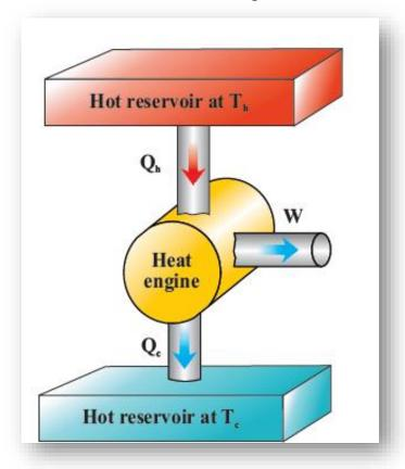
A heat engine absorbs heat  $Q_h$  from a high temperature or "hot" reservoir. It transforms a portion of the absorbed heat into work W, and the rest is given off waste heat,  $Q_c$ , at a relatively low temperature to the "cold" reservoir. energy conservation can be written as follows
