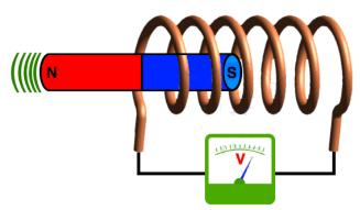
As magnet moves more rapidly to the right, magnetic field is changing more rapidly with respect to the coil and a greater EMF is induced.
