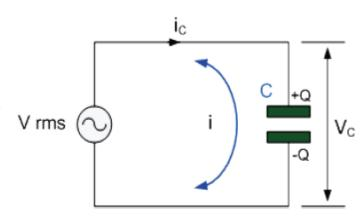
and current flowing in opposite direction, hence capacitor charges and discharges. In this way, the alternating current flows through the capacitor.
