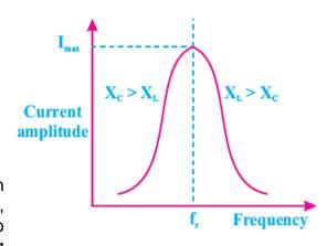
in maximum current flowing through the circuit, moreover either side of the resonant frequency the current in the circuit decreases, as shown in the figure. RLC series circuit is an important circuit it is used in; Electronic filters, Electromagnetic Interference (EMI) Suppression, Tuned Circuits, etc.
