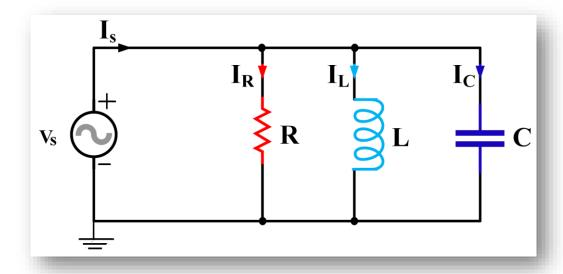
In the above parallel RLC circuit, we can see that the supply voltage,  $V_S$  is common to all three components whilst the supply current IS consists of three parts. The current flowing through the resistor,  $I_R$ , the current flowing through the inductor,  $I_L$  and the current through the capacitor,  $I_C$ .
