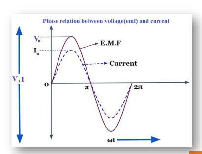
The current  $I_R$  flowing through a resistor R is in phase with the voltage  $V_R$  across the resistor. This alignment can be visually represented on a phasor diagram by depicting a vector (h) that coincides with the voltage  $(V_R)$ .
