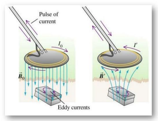
A simplified explanation of the working of a metal detector is described below:
