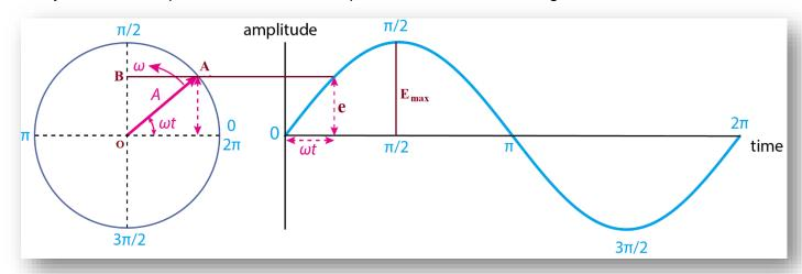
An arrowhead is placed at the outer end of the phasor, serving both to indicate the assumed the direction of movement and to specify the precise length of the phasor, especially when multiple phasors coincide.
