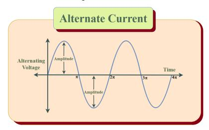
Alternating current (AC) varies in a sinusoidal pattern and follows the shape of a sine wave. This pattern is characterized by a smooth, periodic oscillation that changes direction between positive and negative. While any current that alternates direction could be considered AC, the term typically refers to currents that exhibit this regular, sinusoidal pattern. This sinusoidal nature is fundamental to how AC is generated and utilized in power systems.
