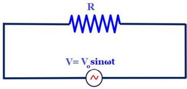
The alternating voltage induces oscillatory motion of free electrons within the resistor, constituting the alternating current. At any given time 't,' the potential difference across the resistor's terminals is expressed as
