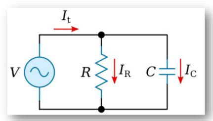
The figure below shows a composite diagram of the circuit conditions. The current phasors  $I_R$  and  $I_C$  are out of phase, therefore, phasor addition must be used to determine the total current. The solving of an RC circuit follows the method previously applied to LR circuits.
