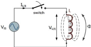
When switch is closed, the current starts to flow. through the inductor, notice that the magnitude and direction of current are changing hence, the associated magnetic field also varies due to which an induced emf is set up in the inductor to oppose the change by the Lenz law. The magnitude of induced emf is given by
