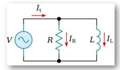
In a parallel DC circuit, the voltage across each parallel branch is equal. This is also true of the AC parallel circuit.
