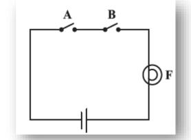
**Behavior**: The lamp will light up only when both Switch A and Switch B are in the ON position. If either or both Switches are OFF, the lamp remains off.
