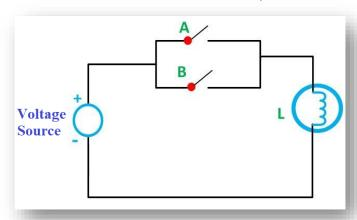
**Behavior**: The lamp will light up if either or both Switch A and Switch B are in the ON position. The lamp remains off only when both switches are OFF.
