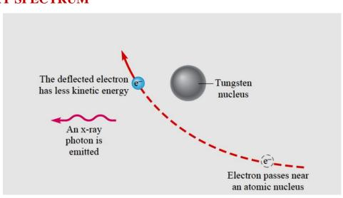
This process is termed BREHMSSTRAHLUNG (German "braking radiation"). The cut-off wavelength  $\lambda_0$  of the continuous spectrum corresponds to the incident in which an electron loses all of its energy in a single encounter with the target atom. The smooth curve
