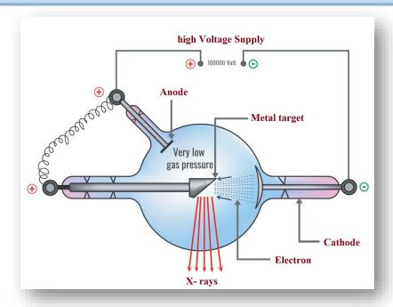
In this tube cathode 'c' is heated by filament "F' and electrons are given off. These electrons are accelerated toward a target 'T' at a very high voltage (several thousand volts). When they strike the target, X-rays are produced.
