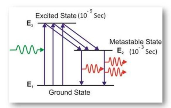
The electrons are excited from ground state  $E_1$  to excited  $E_3$ . The electrons jump from an excited state to the metastable state  $E_2$  whose life is  $10^{-3}$  s, due to the continuous excitation the population in the metal stable state increases then the ground state. This condition is called population inversion which is essential for the production of lasers.
