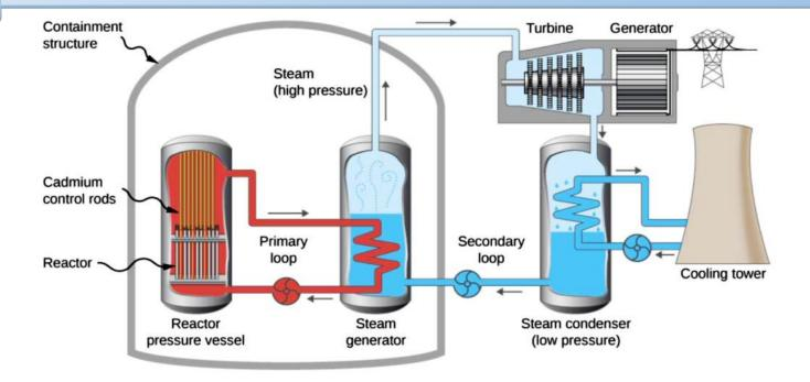
The following are the main components of the nuclear reactor:
