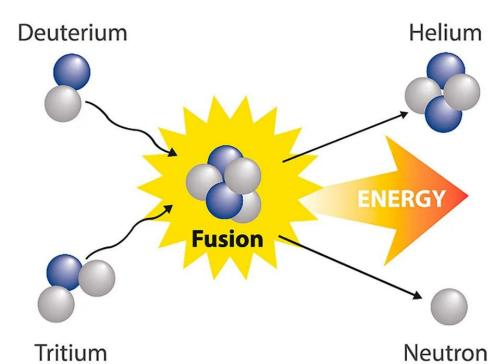
The net result of these two nuclear reactions is that three deuterium  $\binom{2}{1}H$  nuclei fuse together to form a helium nucleus  $\binom{4}{2}He$ ) and a neutron with the release of 21.6 MeV (4.03 + 17.59 = 21.62 MeV). This energy of 21.62 MeV is obtained in the form of kinetic energy of proton
